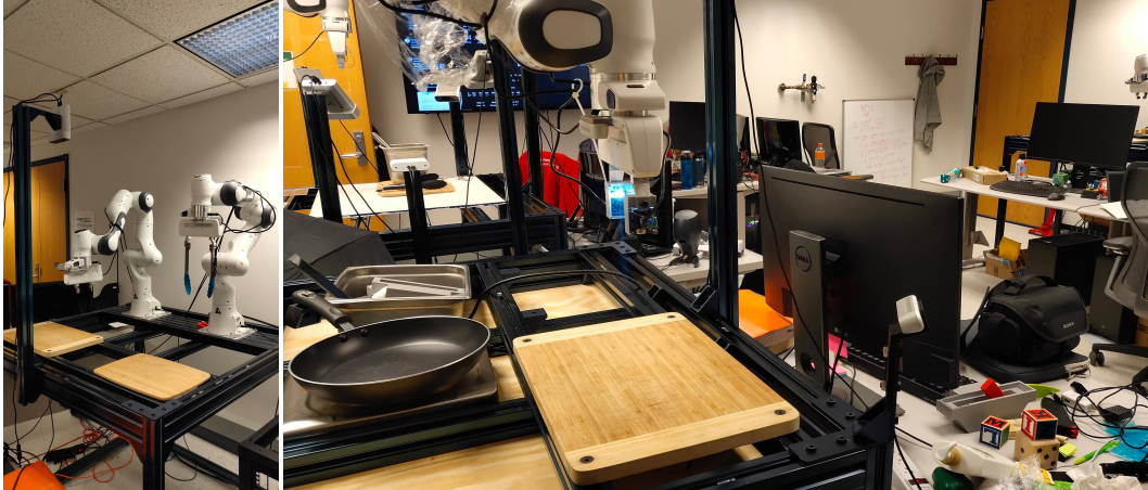
Figure 1: Caption (a) Left: Franka Panda Robot, fitted with custom end-effectors are used to interact differently with various food objects. Azure Kinect setup facing the chopping board is used as the main overhead camera. (b) Right: Finger-vision camera setup, as seen on the end-effectors. Realsense cameras mounted at different points to capture depth information.
